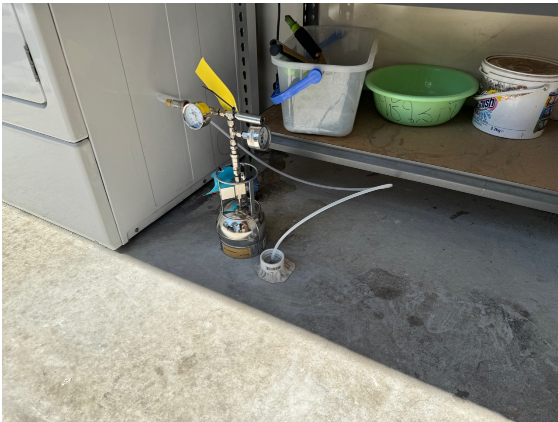
Photograph 10: Soil vapour sampling setup that was completed in the area the subject of the former NSW EPA Clean-up Notice.
